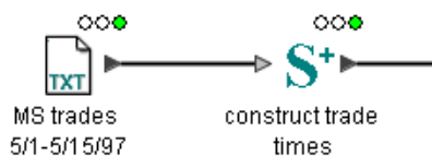
Figure 1: An S-PLUS Script node used to convert separate time and data columns into a single column containing both time and date information.
